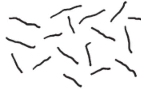
(b) Map cracking.
